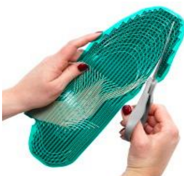
Figure 15 Sensor being cut according to requirement
